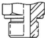
DIN 3852 Form B: Sealing by means of a sealing "shoulder." Female thread is parallel.
