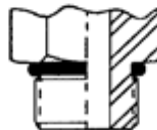
Form SAE J514: Sealing by means of an O-Ring in the thread undercut. Female thread is parallel.
