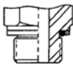
DIN 3852 Form A (formerly Form D): Sealing by means of a washer or bonded seal. Female thread is parallel.
