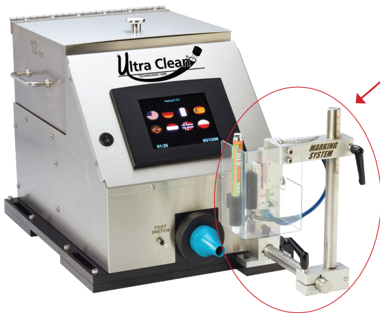
UC-CAL-MARK in place on UC-CAL-G1.5 Carousel AutoLoader
